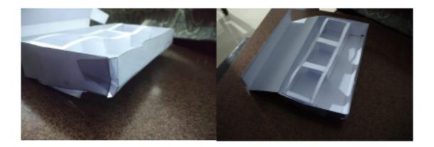
With the limited resources we have at home we tried to experiment with paper and cardboard to study the form and flding techniques to make a design which can be folded to a box from a plane sheet of cardboard.
