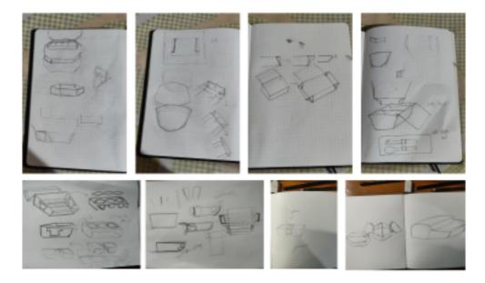
We went forward with another set of ideation by removing the handle flap. We tried new ways like a flap, which can be pulled down from the base to act as the side walls when placed on a lap, and one where at shape is pushed down, and it falls to form the side walls.
